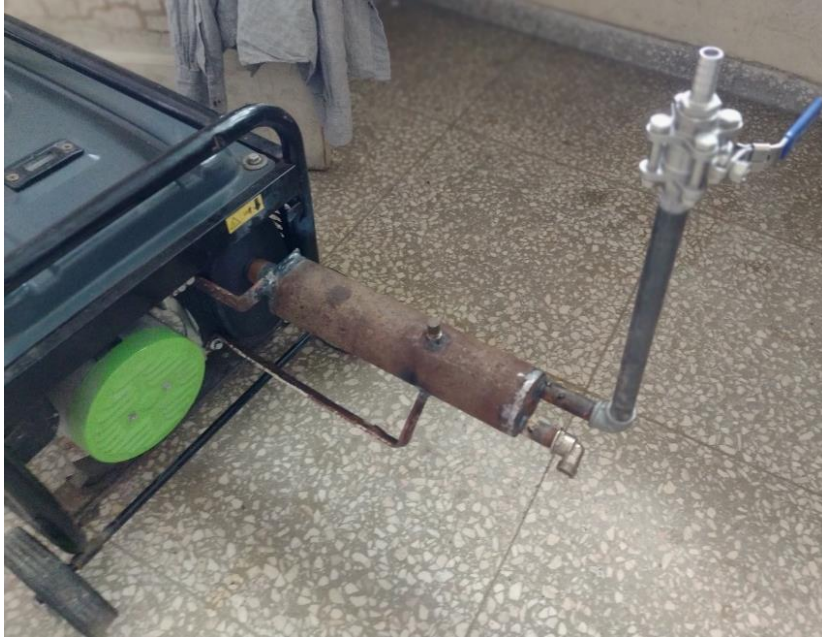
Figure 19: Misaligned bars welded on Manifold (Source: Own Work)
