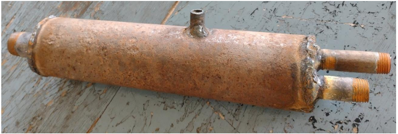
Figure 17: Manifold Side View (Source: Own Work)
