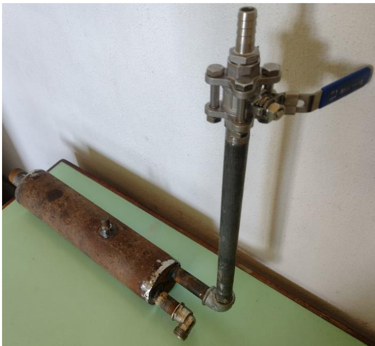
Figure 18: Manifold with Ball Valve ((Source: Own Work)
