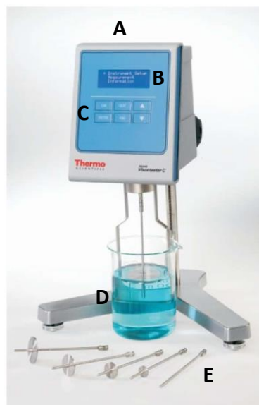
Figuur 1 HAAKE Viscotester D type R Bron: HAAKETM ViscotesterTM E, D and C Rotational Viscometer, 2020
