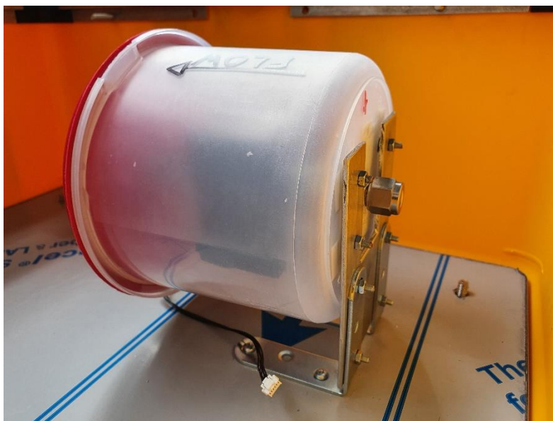
Figure 33 Fixing the OPC-N3 box to the bottom case panel
