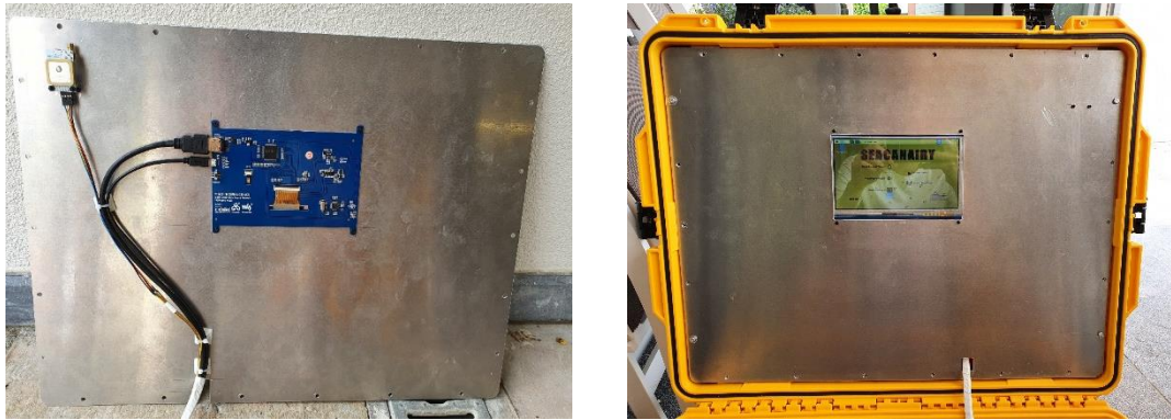
Figure 25 Cover plate (in the case lid), back and front side
